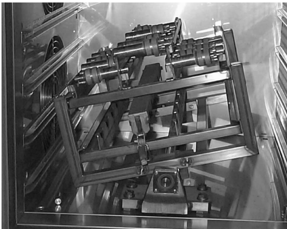
Fig. 2. Multiautoclave device utilised during explorative zeolite synthesis.
